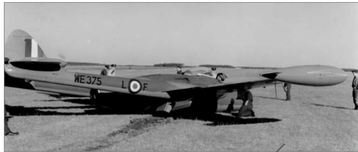
After the undercarriage refused to lower the pilot of WE375 L-F of 98 Sqn pulled off this successful wheels up landing at Fassberg in early 1954. The Cat.3 damage was soon repaired and '375 continued to fly with 98 and 145 Sqns. (Brian Sharman)
