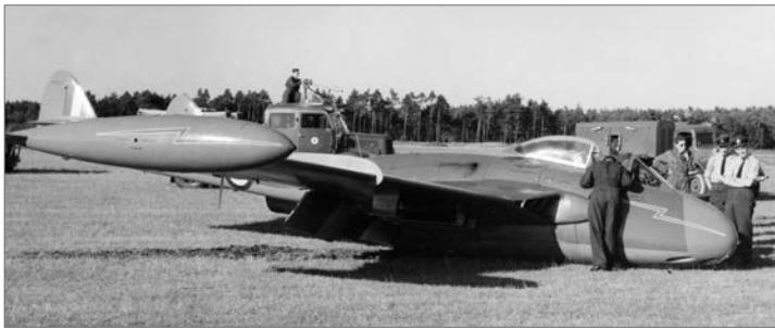
After the undercarriage refused to lower the pilot of WE375 L-F of 98 Sqn pulled off this successful wheels up landing at Fassberg in early 1954. The Cat.3 damage was soon repaired and '375 continued to fly with 98 and 145 Sqns. (Brian Sharman)
