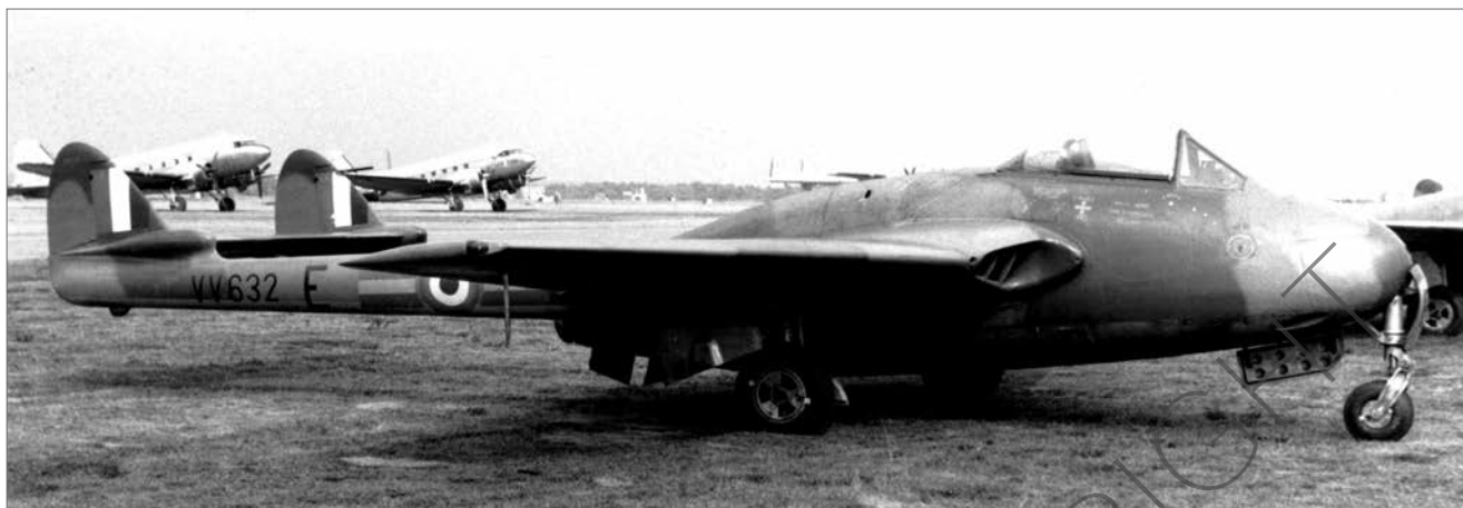
Original FB.5 engine air intake shown on VV632/E of 613 Sqn in 1955. (MAP)
